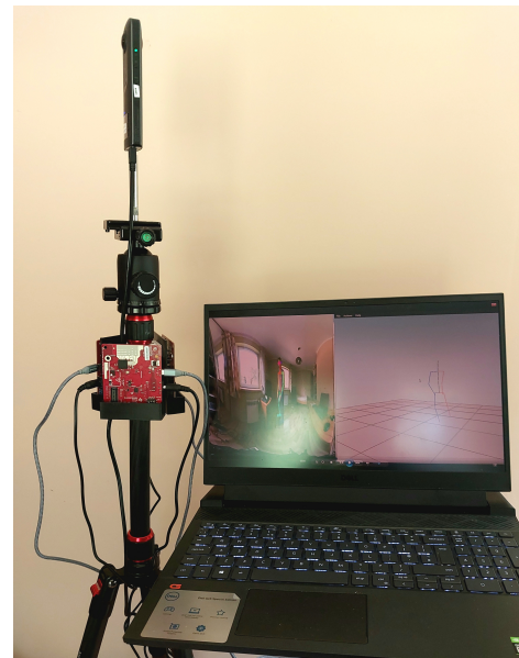
Fig. 1. Our experimental setup consists of a laptop with RTX 3060, the Ricoh Theta V omnidirectional camera and three TI AWR1843BOOST mmWave radars.
